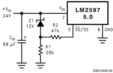
**FIGURE 31. Undervoltage Lockout for a Buck Regulator**
