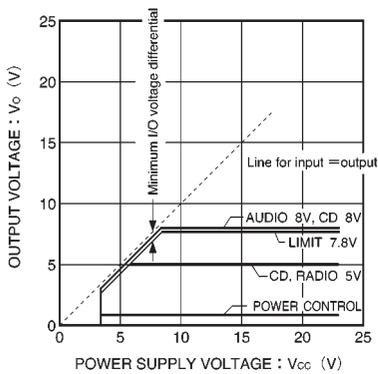
Fig.2 Output voltages vs. power supply voltage
