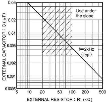
Fig. 8 Value of external components for oscillator
