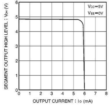
Fig. 10 Segment high level output vs. output current
